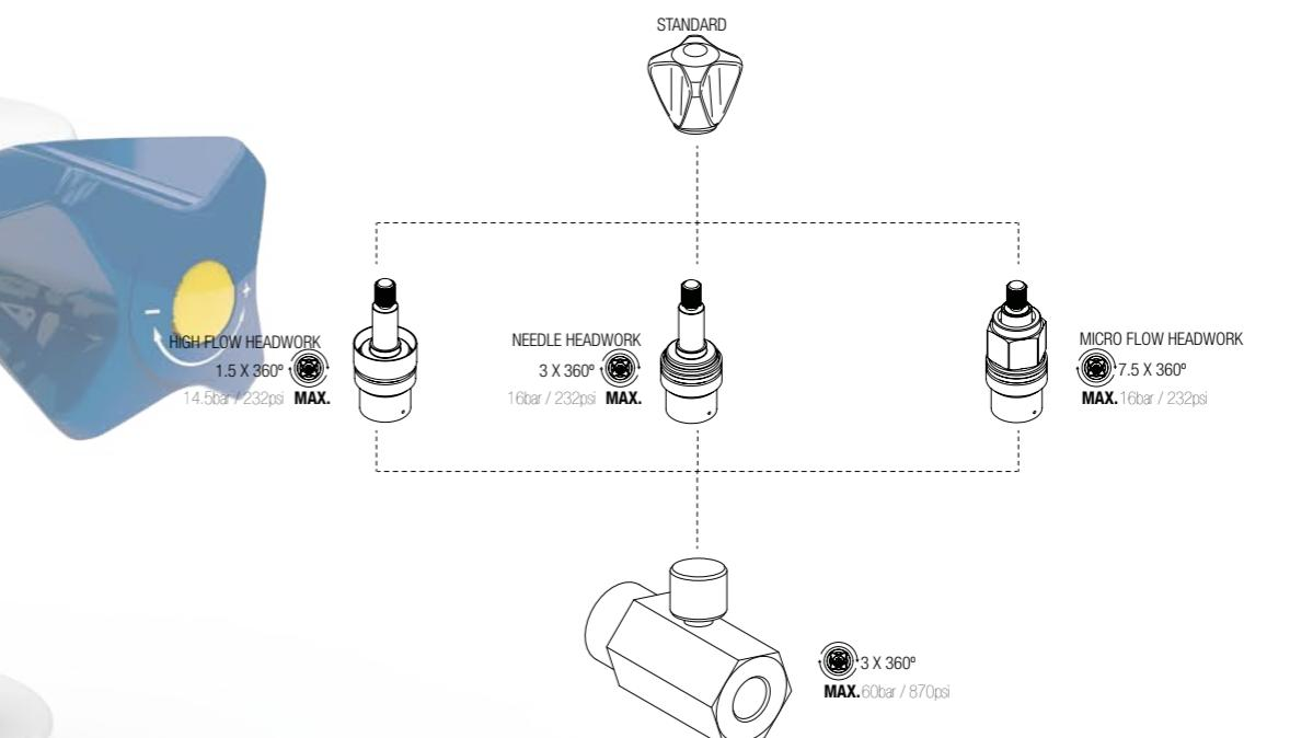
FLOW VALVE WITH OUTLET: FEMALE 1/4" NPT
